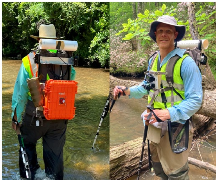
Figure 2: HDSS backpack setup for the survey on wadable segments of Parkerson Mill Creek. Emlid Reach M2 was located at the top of the backpack directly behind the surveyor's head on the backpack. Two video cameras were located on the chest of surveyor (forward and down views) and two cameras were mounted on the left and right of the backpack frame providing a view of the left and right streambanks. A GPSMap 64 was also located in the front breast pocket of the surveyor.
